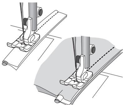
Insert packaged piping into seams and edges for a tailored finish. Cover cord with fabric for specialty piping. The clear view allows you to see the piping placement and see exactly where you are stitching. The clear view enables you to see the first row of stitching and adjust your needle position to stitch next to the original row. Straight Stitch, length 2.5.
