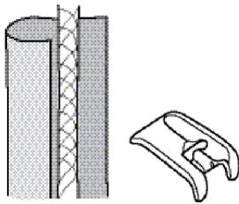
4. Place the fabric and cord under the Single Welt Cord Foot with the cording in the groove on the underside of the foot.
