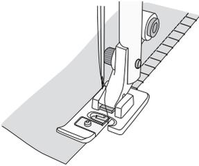
The J Foot is used for overcast stitches that stitch to the side and can pucker or curl the fabric to prevent the fabric from curling under. The tiny wire on the edge of the foot prevents the curling of the fabric edge. Consult the HUSQVARNA® VIKING® Infodisplay which recommends the J Foot for many overedge stitches.
