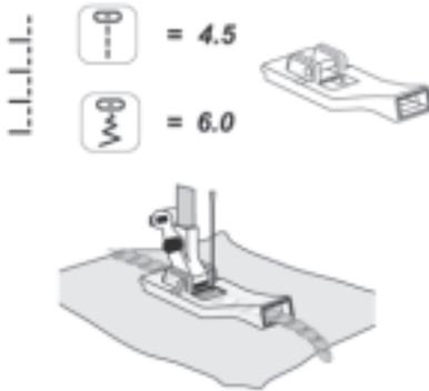
1. Thread with invisible thread on top and regular sewing thread in the bobbin. Snap on the Fancy Trim Foot and select a Hand Look Appliqué Stitch. Adjust the stitch length to 4.5 and the width according to the width of your sequins. Make sure to use Tear-Away stabilizer underneath your fabric.
