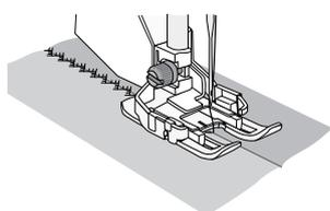
The Interchangeable Dual Feed with Changeable Presser Feet is designed to feed layers of fabric and/or batting evenly. It is perfect for quilting, sewing velvet, some stretch fabrics, imitation leathers and fabrics which need accurate pattern matching. Use the Changeable Open Toe Foot when sewing Satin stitch applique, Taper stitches and Decorative stitches. The tunnel on the underside of the foot feeds smoothly and the open front gives greater visibility and a great overview of the stitches.
