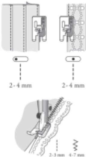
1. Snap on the Edge/Joining Foot.
