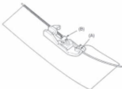
This foot is used for sewing yarns (cords, nylon gut) up to a thickness of 1.0 mm. This produces an undulating or stiffer hem (e.g. on wedding dresses and valance).
