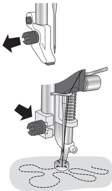
1. Loosen the presser foot ankle screw completely and remove the ankle.
