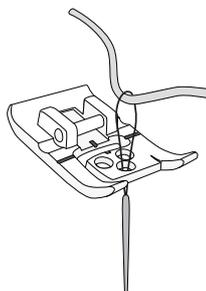
Embellish your project with different types of decorative cords or yarn using beautiful HUSQVARNA® VIKING® 9 mm stitches and the Three Hole Yarn Foot. This foot will easily guide the cords or yarn through the openings in the front of the foot back through the groove under the presser foot. The decorative cords or yarn will be stitched over creating a beautiful braid embellishment.
