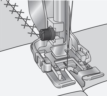
The Interchangeable Dual Feed with Changeable Presser Feet is designed to feed layers of fabric and/or batting evenly. It is perfect for quilting, sewing velvet, most stretch fabrics, imitation leathers and fabrics which need accurate pattern matching. Use the Changeable Decorative Guide Foot when stitching in the ditch along a seam line sewing any decorative stitch. The metal guide in the center of the foot helps you when guiding your fabric.
