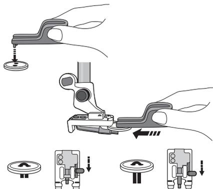
This presser foot for sewing on buttons raises the button slightly off the fabric to give a slight thread shank to enable easy buttoning, and prevent the button from being sewn too tightly to the fabric.
