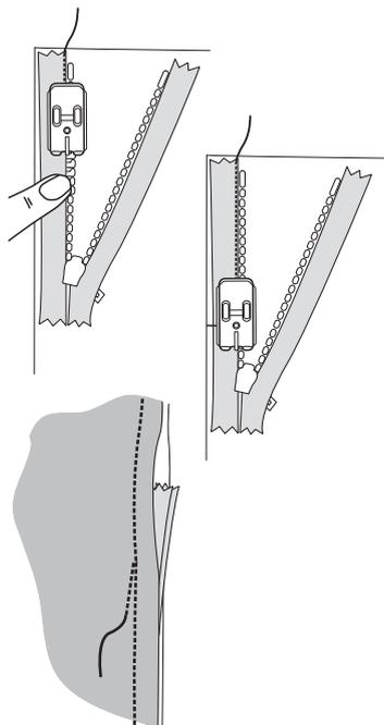
1. Mark the length of the zipper opening on the seam allowance and on the zipper. The excess length should be at the bottom of the zipper. Snap on the Invisible Zipper Foot. Select center needle position straight stitch. Length 2.5–3.0.
