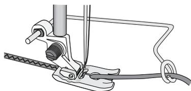
1. Thread braid from top of foot into the guide hole and under the foot.
