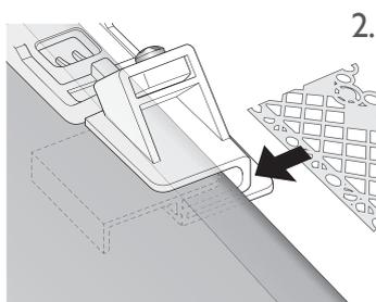
**Note:** Adjust the screw on the guide to adjust the stitch position if needed.
