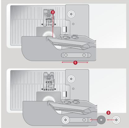
The Double Fold 1/2" (12mm) binder will turn a light weight woven fabric strip into a binding and attach it to the project edges all in one step when fitted with 412964206 or 412964207 stitch plate.
