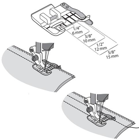
The Seam Guide Foot for IDF™ system guides your stitching perfectly when joining fabrics. The presser foot is designed to help you keep the seam allowance at the same distance from the edge throughout the project. The presser foot has a metal guide at 5/8 inch distance from the center needle position, which is the most used seam allowance when sewing clothes. It has four more markings for various seam allowances.
