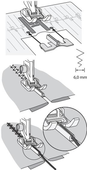
1. Snap the Distance Plate onto the needle plate by placing the little prongs into the holes in the plate. Be sure that the plate doesn't cover the feed teeth. Snap on the Spanish Hemstitch Foot.
